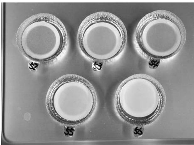
Fig.6 The paper filter in the SS measurement
